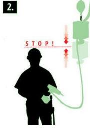
THE POSITIONER HOLDS THE APPLICATION AUTOMATICALLY AT THE DESIRED HEIGHT. HOLDS THE APPLICATION, EVEN IF THE LOAD WEIGHT CHANGES.
